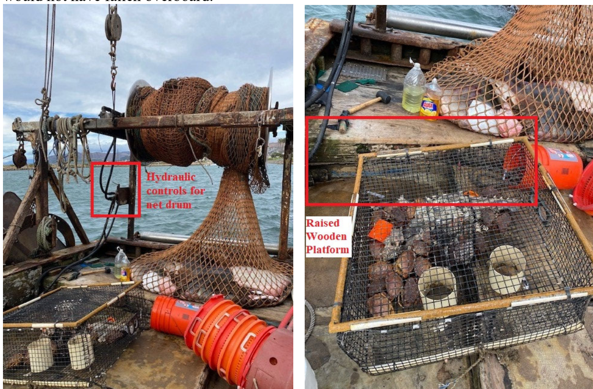
Figures 6 & 7: Hydraulic control location / raised wooden platform (vessel's last known configuration).
