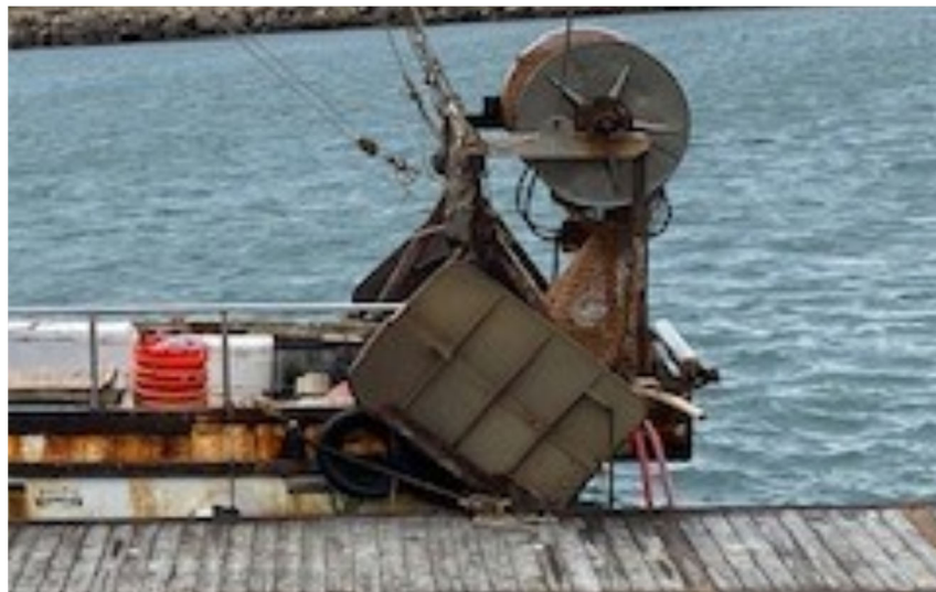
Figure 4: Close-up view of stowed metal fishing doors, portside.
