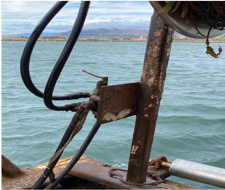
Figure 5: Hydraulic lever operating the fishing net drum.
